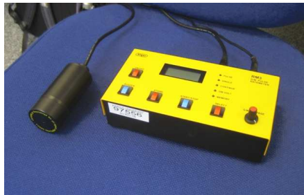
(a) Geiger-Müller tube (left) and pulse ratemeter with data log and serial interface (right)
